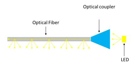
The optical fiber is treated in order to let the light escape through thousands of "holes". This phenomenon generates a smooth, non-aggressive, warm light.
